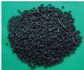
FIGURE 1. Carbon molecular sieve (CMS) pellets, typically manufactured from coconut shells, provide the surface area and pore structure needed to separate oxygen and nitrogen from a compressed air inlet stream
